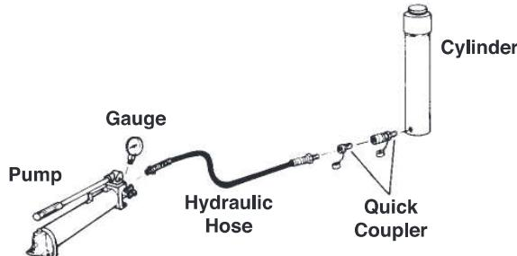
Since the single-acting cylinders have only one hose going to the cylinder, the cylinder can only apply force to extend (pull cylinders retract) its rod. The return stroke is accomplished by gravity or spring force.
