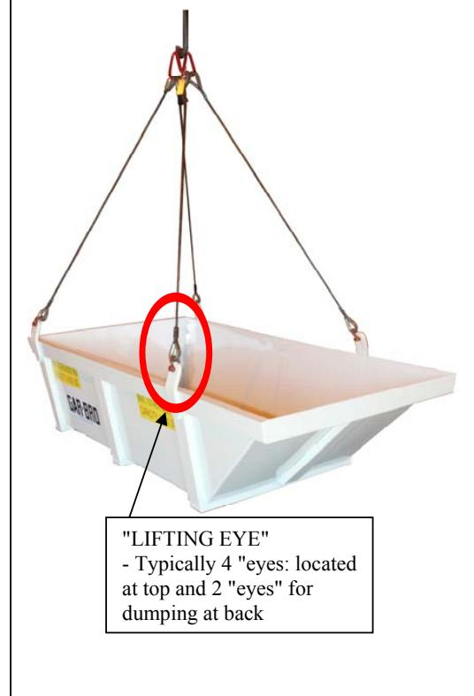
anchor shackles, etc.) should be inspected daily for fraying, damage, and wear and must be immediately removed from service if deemed unsafe.
