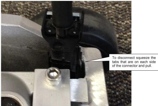
3. Remove the cover plate(if one piece). If the two piece top cover, only the small cover needs to be removed.
