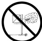
Never operate during high wind conditions. Lifting bulky loads during high winds can result in the lift tipping over and the possibility of operator injury.
