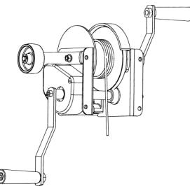
10. Wind the slack cable tightly and evenly across the load drum.
