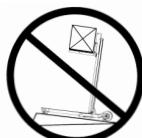
Operate only on level surfaces. Use the unit on smooth and level surfaces to avoid unit tipping over and the possibility of operator injury.
