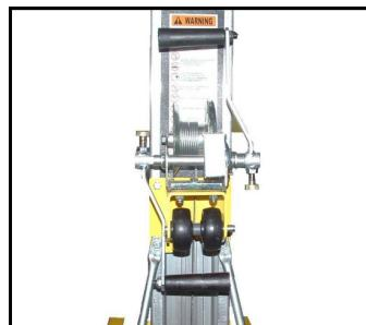
The winch handles have been placed in the stored position.
