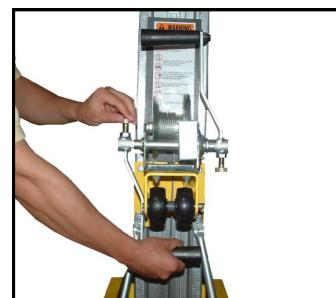
To place the winch handles in the operating position, pull up on the locking pin and slide the handle off of the winch shaft. Rotate the handle assembly around so that the black plastic grip is facing away from the winch. While pulling up on the locking pin, slide the handle back on to the winch shaft. Repeat this procedure for the other handle.
