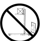
Keep work area clean. Always keep work area clear of clutter for unobstructed movement of the unit. Never leave elevated load unattended.
