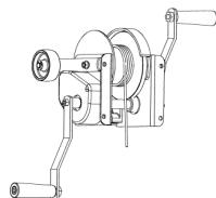
If cable is kinked, worn, frayed, damaged, or has anything on it that would obstruct its rotation around the pulley wheels, **do not use the unit!**
