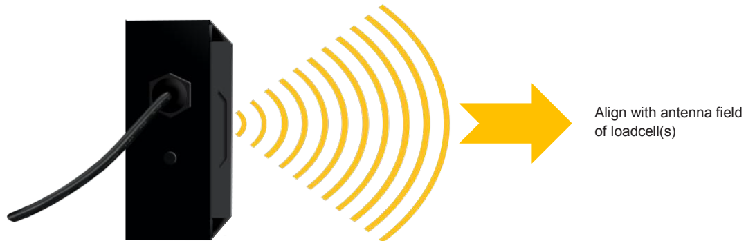
Fig. 3 Establishing an obstacle free line-of-sight path between the USBBE receiver and the loadcell transmitter will provide best quality radio link and greatest range.
